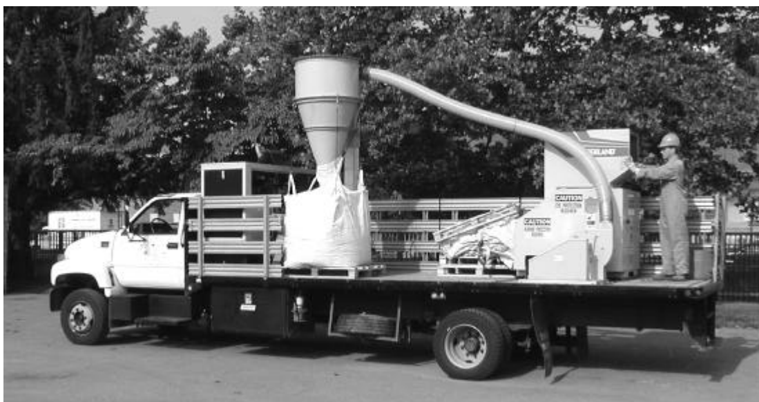
The Pennsylvania Dept. of Agriculture's new granulator reduces mountains of containers to bags of chips.
